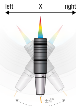
3 Max. tilt angle in X \pm 4^\circ
