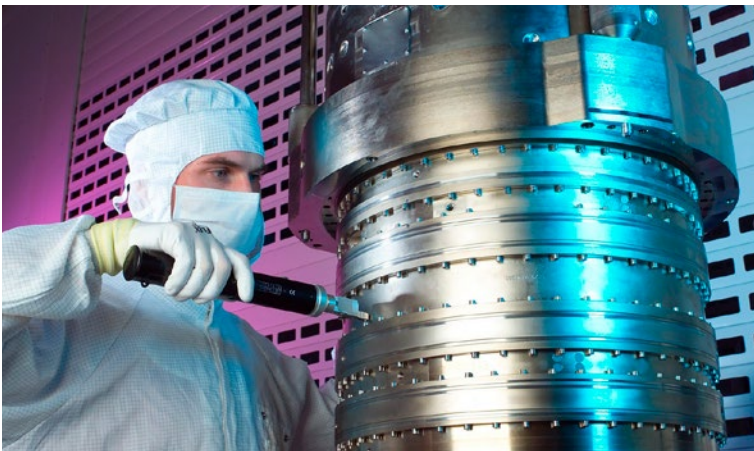
Capacitive displacement sensors are used for adjustment with nanometer precision of lenses in optical systems for wafer exposure.
