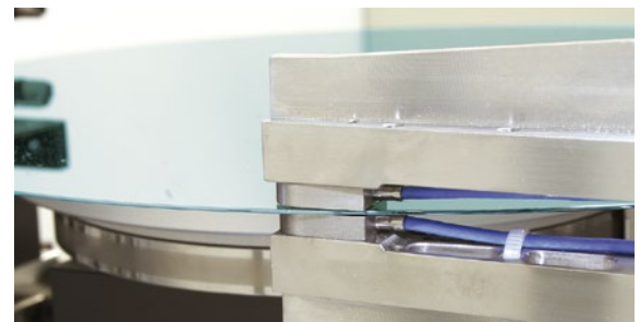
Wafer thickness measurement with two capacitive sensors
