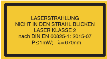
Fig. 1 Laser labels on the sensor cable
