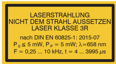
Fig. 4 Laser labels on the sensor cable
