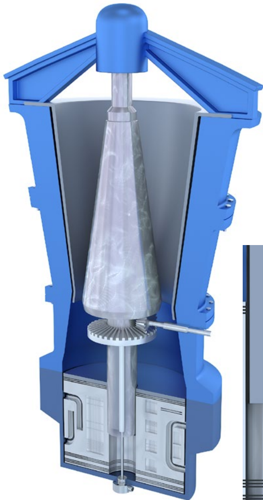
EDS-F: Measuring the grinding gap in crushers
